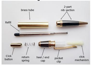
You will require a blank at least 56mm long drilled out to 10.7mm. Once the brass tube has been glued into the drilled blank it can be turned using a bushing set either on a mandrel or between centres as you prefer. There must be NO GLUE inside the tube or it may foul the mechanism and prevent the pen from working correctly.
